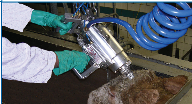
Non-penetrating stunner used with monorail restrainer.
